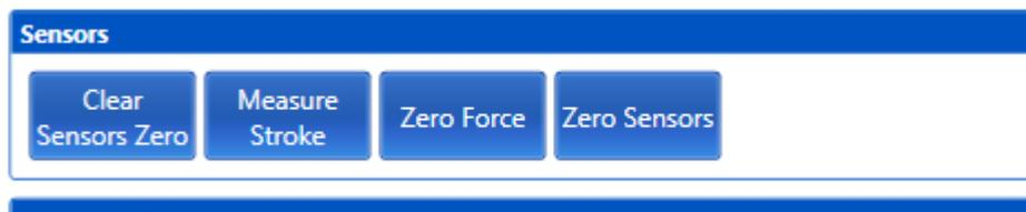
Sensor commands tells the software to do something with sensor data before or during the test. For most tests, none of these commands would be used during a normal test.
